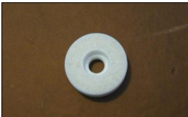
Fig. 6: Customized Teflon Block with a Central Cylindrical Through Hole
