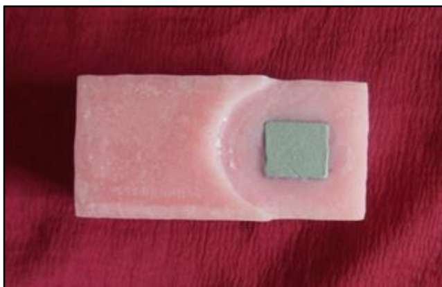
Fig. 5: Metal Plate Embedded in Acrylic Block
