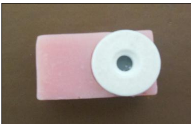
Fig. 7: Teflon Block Placed on Metal Plate Embedded in Acrylic Block
